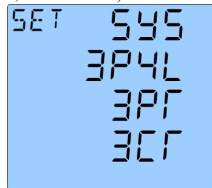
Figure 3.3.2.6 system wiring setup page
