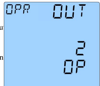
Figure 3.4.2.5 second relay operation
