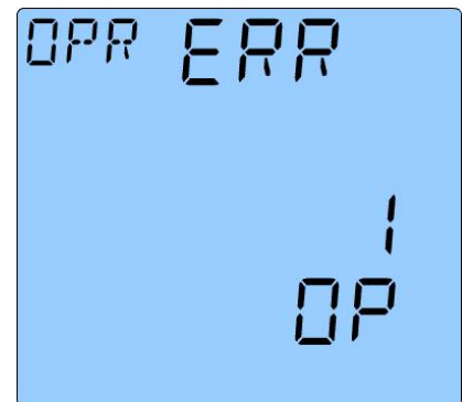
Figure 3.4.2.4 relay local operation fails
